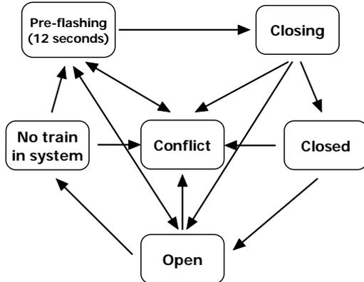
Fig.5. Graph of the level crossing's control object
